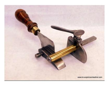
Plough gauges are a European strap cutting tool. These have a handled blade that is pushed into the leather and the guide is on the left side. These have likewise been around a couple hundred years in several versions.
