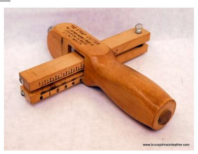
The wooden strap cutters are pretty commonly found and used. They have a wooden handle, two parallel bars that support a blade, and adjust up to 4 inches wide. They use a replaceable blade – with
