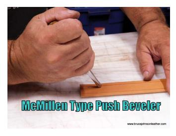
I was taught to use a push beveler that is repurposed from a single line creaser. I make these up in the shop myself from creasers. The working end is ground to a smooth face at angle with the steep either to the right or left side. The face is polished smoothly. Some users will want the steep angle to be on one side or the other depending on how you prefer to use it.
