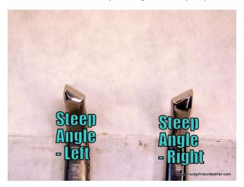
I am right handed and leaning over the piece, I prefer the steep angle to be on the right side and bevel the left side of the cut line. I was taught to hold the tool in my right hand and lean into it with my elbow at my side as I push it forward. The first pass is light to establish the bevel. On additional passes I lean into the tool with more force to make a more distinct bevel.
