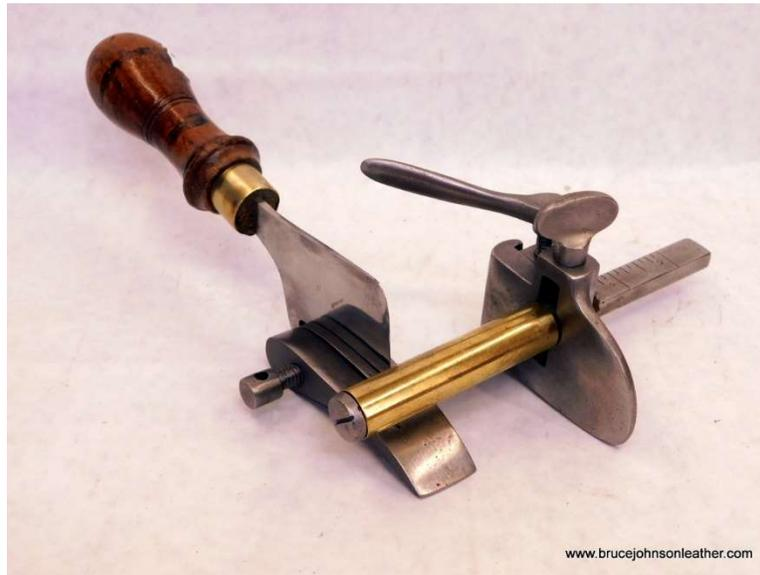
Plough gauges are a European strap cutting tool. These have a handled blade that is pushed into the leather and the guide is on the left side. These have likewise been around a couple hundred years in several versions.
