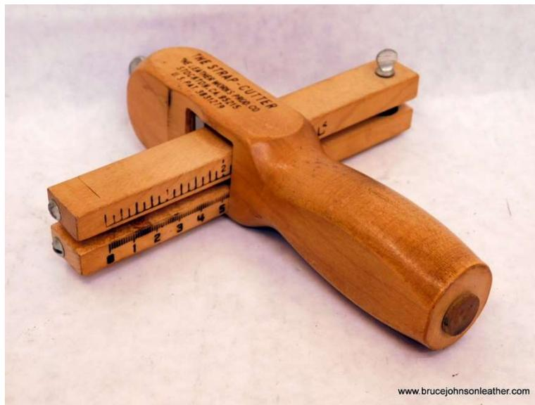
The wooden strap cutters are pretty commonly found and used. They have a wooden handle, two parallel bars that support a blade, and adjust up to 4 inches wide. They use a replaceable blade – with
