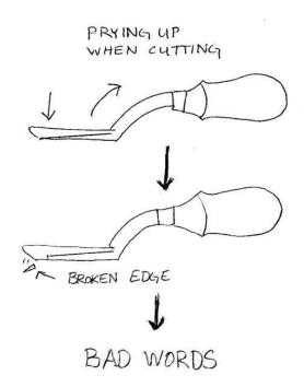
The other big concern is maintaining the edge. Strop the edge as you would a knife and the edge will last quite a while. You are cutting a lot of leather with a narrow section of blade and some routine maintenance makes the French edger a friendly and useful tool.
