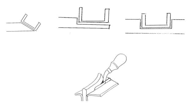
Sharpening – There are a few ways to sharpen a French edger and some are diametrically opposite to achieve the same result. To further compound the issue, there are two kinds of edges on French edgers. Most of the older French edgers were made with a thinner blade stick area and result in a thin edge, much like a thin knife edge. Others are made from thicker stock, flat on the bottom with an angled bevel on the top edge like a chisel.
