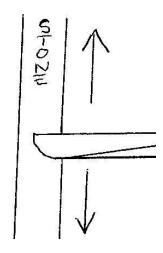
Once I have the square leading edge, then I begin to bring an even bevel across the entire cutting edge. I was taught to mostly work off the bottom. I do that by pushing the tool into an appropriate grit sharpening stone or wet-dry sandpaper on a flat surface. On the curved bottom edgers you need to pay special attention to doing an even stroke and contact on the length of the bottom surface .
