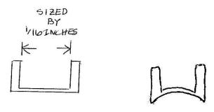
Sizing – French edgers are sized by the width of the cutting edge between the side rails. The common size pattern seems to be that each number is 1/16 inch wide,, i.e. a #3 French edger cuts 3/16" wide.
